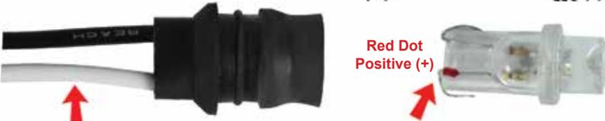
Some of these LEDs are replaceable, if any were to burn out you can replace them easily.
